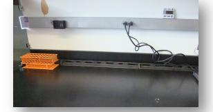
The URB is fastened to the bench top with a strong 3M adhesive strip.
